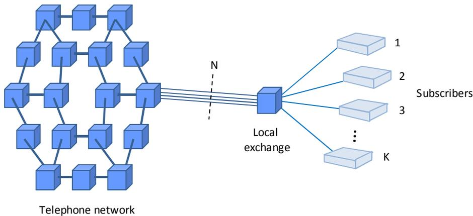
**Figure T.3:** Subscribers connected to the telephone network via access lines.
