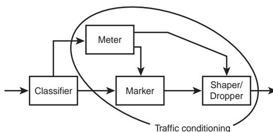
A traffic profile is one way to present the traffic-conditioning rules. In the simplest model, each packet is either *in-profile* or *out-of-profile* based on the metering result at the arrival time of the packet. In-profile packets obtain better traffic-conditioning and forwarding treatment than out-of-profile packets. This model is further evaluated in this book in section 7.4, “Assured Forwarding PHB Group,” of Chapter 7.
