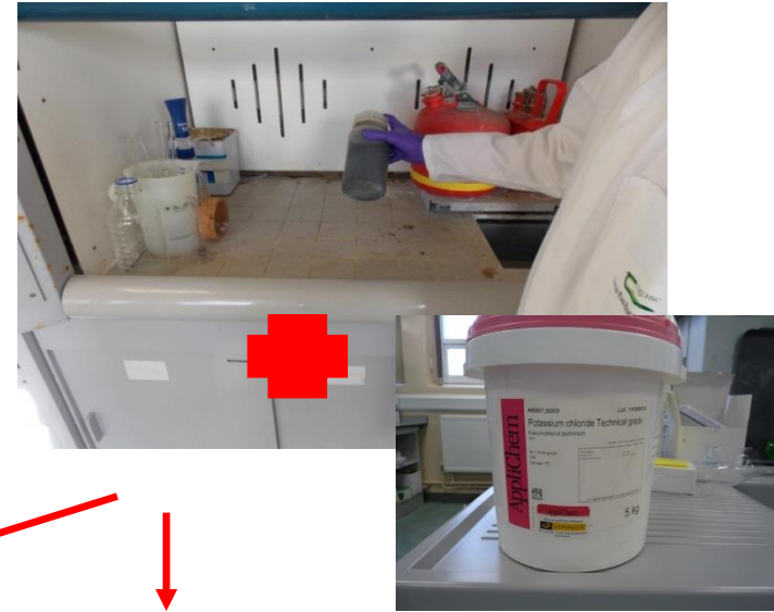
Shaking sample with KCL extractant
