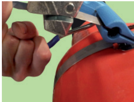
6. To loosen the tape with the crank lever a little bit at the same time, bend tape at maximum tension (about half a turn). Cut tape with cutting crank after wards.
