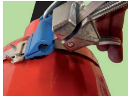
4. Fix tape with the blocking lever
