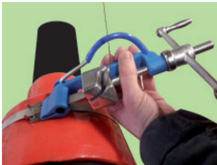
5. Afterwards stretch tape with the crank lever
