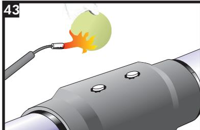
Heat the adhesive side of the CFS with a medium intensity flame until the adhesive becomes glossy (Adhesive will melt).
