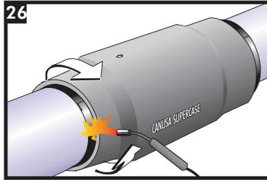
Using broad strokes and a medium flame, begin shrinking one end of the CSC evenly all around. Keep the torch moving to avoid overheating any spots; ensure sufficient heat is applied at the bottom.
