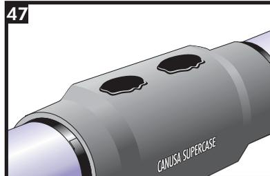
The CFS has been fully installed when adhesive can be seen around the entire circumference and is in full contact with the casing.
