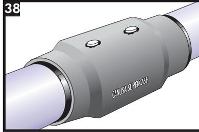
Visually inspect the completed casing. **Ensure that the ends of the CSC are completely shrunk down.** To double seal the foaming hole use a Canusa Foam Seal - CFS.
