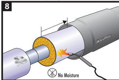
Use a propane torch with a low flame to dry the jacket pipe, carrier pipe and CSC. Use a dry, grease and lint-free rag to wipe clean the jacket pipe, carrier pipe and CSC.
