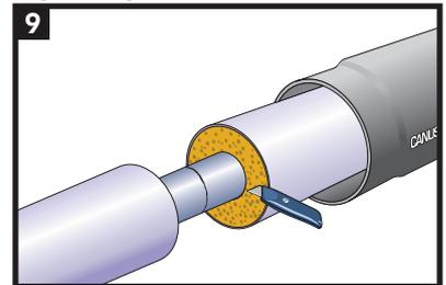
Remove any wet PUR foam from the end of the pre-insulated pipe.
