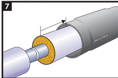
Check the CSC to ensure that it is not damaged. Before welding together the carrier pipes, slide the CSC as far away from the joint as possible.
