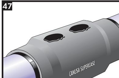
The CFS has been fully installed when adhesive can be seen around the entire circumference and is in full contact with the casing.
