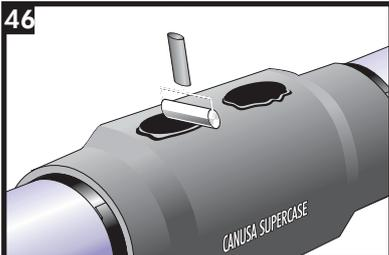
Using a roller, gloved hand or the side of the larger end of the CFS Rolling Tool: smooth out the CFS surface. Ensure adhesive has oozed from all sides of the CFS.
