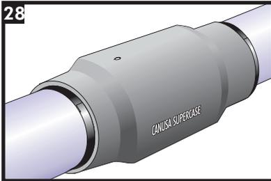
Continue heating the edge until it is fully recovered around the entire circumference of the jacket pipe. **Shrinking has been completed when the shrink zone of the CSC has conformed to the entire pipe jacket.**
