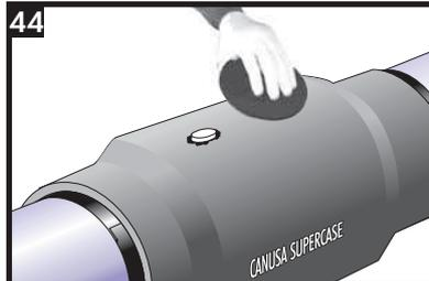
Place the CFS onto the pre-cleaned and pre-warmed section of casing directly over the centre of the foaming hole.
