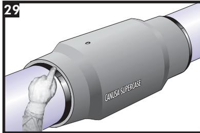
As a final check, ensure that the shrink zone of the CSC conforms intimately with the entire pipe surface. This can be checked by feeling the edges all around the circumference of the casing. If there is edge lifting, the edge should be reworked with additional heat.
