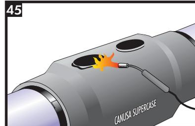
Using a weak medium flame, heat the backside of the CFS until the adhesive oozes from the edge and the thermochromic ink print disappears. **Do not overheat the surface as the foam will gas.**
