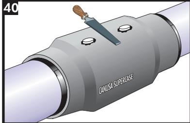
Using a grater, sand down the plugs bringing them flush to the surface of the CSC.
