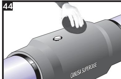
Place the CFS onto the pre-cleaned and pre-warmed section of casing directly over the centre of the foaming hole.
