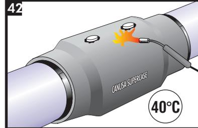
Pre-warm the casing surface around the foaming hole to 40°C. **Do not overheat the surface as the foam will gas.** Check the temperature using a temperature measuring device.
