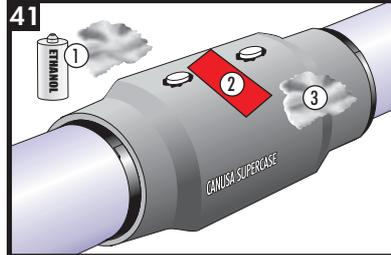
1. De-grease the surface around the plug using a grease and lint-free rag soaked in ethanol.
