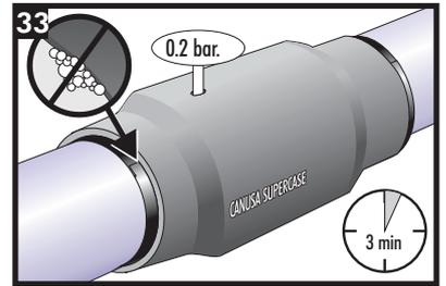
Ensure the CSC shrink zones have cooled to below 40°C. Perform the pressure test using the previously drilled pressure hole. The CSC should be checked with an air pressure test for 3 minutes at 0.2 bar. In case of a leak, the CSC shrink zones should be reworked with additional heat at the leaking area. The pressure test should then be repeated.
