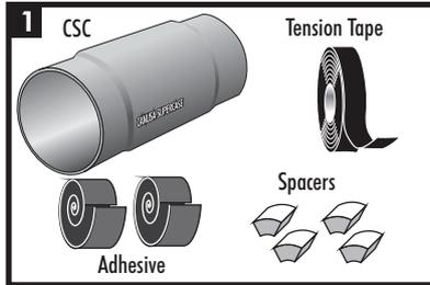
The Canusa SuperCase™ - CSC is a crosslinked, heat shrinkable casing for joint protection of pre-insulated pipe. If the packaged kit is used, it contains: adhesive, spacers and tension tape for large casings.
