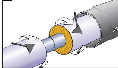
Using a triangular scraper, clean the edges of the jacket pipe to remove any burrs and dirt from the sealing area.
