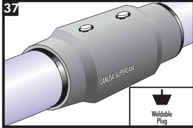
After the foam has hardened, remove the ventilation plugs and drill any holes necessary for sealing. When using Canusa approved weldable plugs and welding machine, it is required to match the conical geometry with all pieces of equipment (i.e. weldable plug, drill bit, welding machine heating cups). **Cylindrical tools for plug welding are not recommended.** Note: Using an approved welding tool, (at 250°C) the recommended times for plug welding are:
