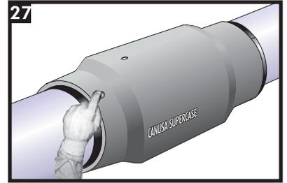
With a gloved finger, press down on the shrunken area to ensure the backing and adhesive are soft. If there are cool spots, the shrink zone should be reworked with additional heat.
