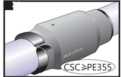
For casing sizes PE355 and above, wrap the supplied tension tape around the edge immediately after shrinking, while the casing is still soft (if the casing has cooled down; reheat it). **This ensures even cooling and conformance of the edges.**
