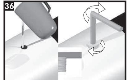
Ensure the CSC shrink zones have cooled to at least 40°C. If they have not, follow the cooling instructions as described in step 31 (for CSC 560 and greater, follow steps 31 and 34). **Do not foam if the surface temperature is above 40°C.** Foam the joint according to the manufacturer's guideline. Use standard ventilation plugs while foaming. After the foam has cured, remove the foaming straps (if used).
