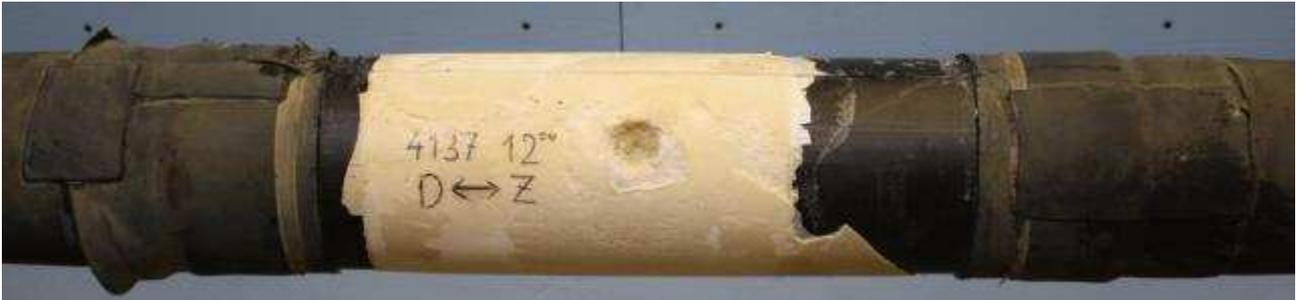
**Figure 4** Destructive test after withdrawals from water tank in the 12-o'clock position (sample 4137, DN 80/160), pull side (Z), compression side (D): dry.
