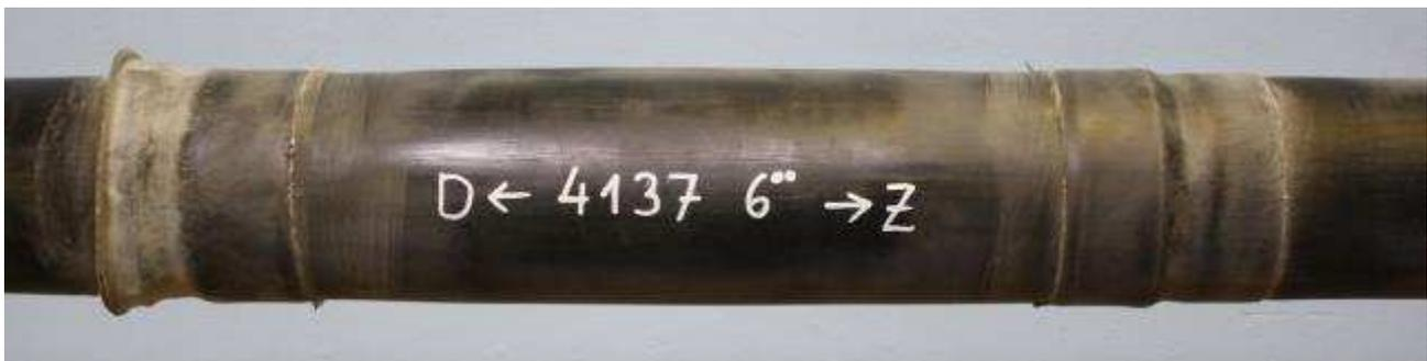
**Figure 3** Joint 4137 after soil stress test in the 6-o'clock position, pull side (Z), compression side (D).
