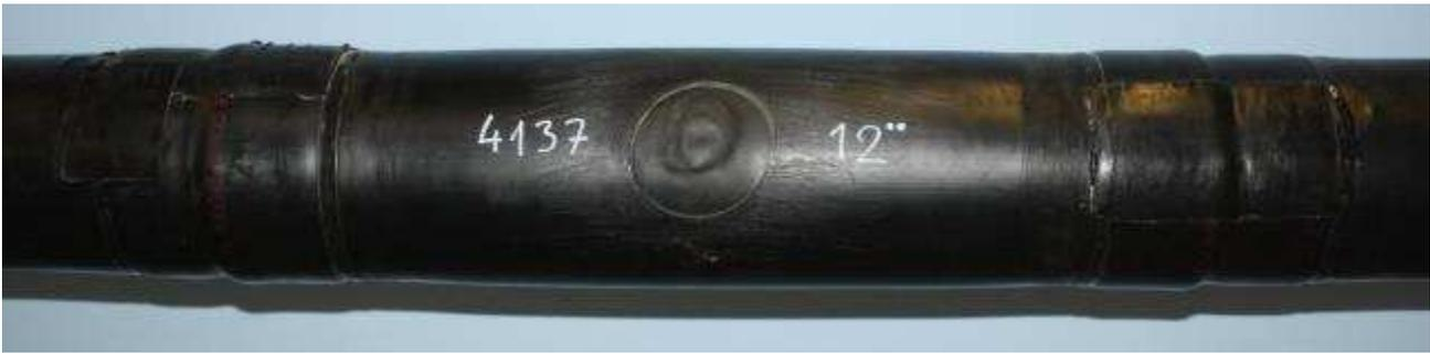
**Figure 1** Joint before the start of the test (sample number 4137, DN 80/160).
