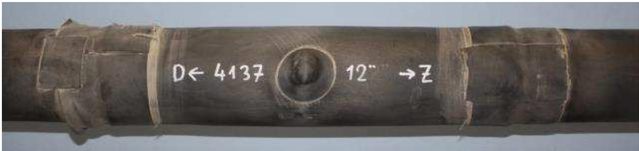
**Figure 2** Joint 4137 after soil stress test in the 12-o'clock position, pull side (Z), compression side (D).
