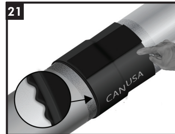
After shrinking, press down on the sleeve to ensure adhesive flow over the entire surface. Special attention should be given along the circumference between 4 and 8 o'clock and along the overlap area. In order to avoid a channel formation at the step down, the sleeve should be pressed down. The shrinking has been completed when an adhesive ooze begins at the sleeve edges all around the circumference.
