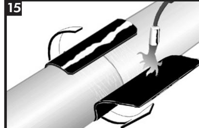
Wrap the sleeve loosely around the pipe, ensuring the appropriate overlap. Gently heat the backing of the underlap and the adhesive side of the overlap.
