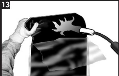
Partially remove the release liner from the sleeve (~15 cm from the edge) and gently heat the adhesive along the underlap with a torch.
