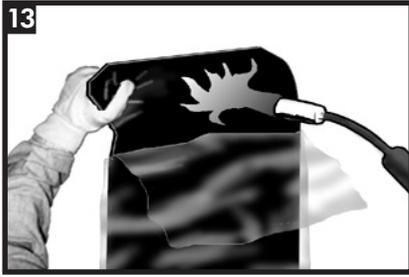
13 Partially remove the release liner from the sleeve (~15 cm from the edge) and gently heat the adhesive along the undertap with a torch.
