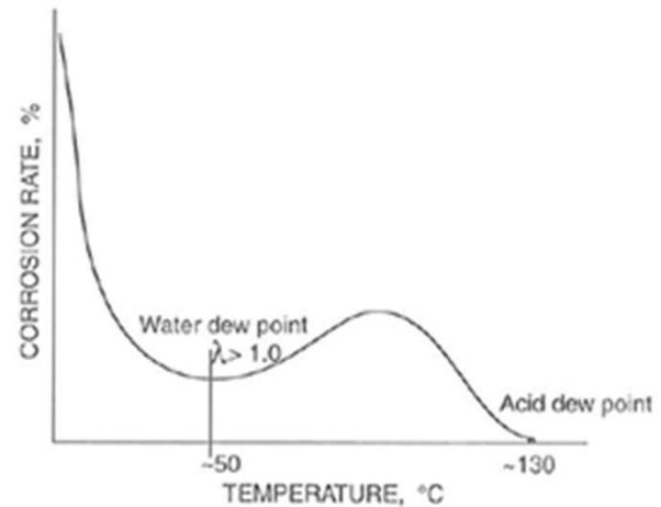
Effect of flue gas temperature on the acid corrosion of heat delivery surfaces.
