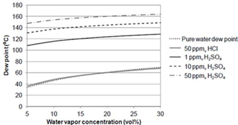
Pure water and sulfuric acid dew point temperature as a function of water vapor concentration in a flue gas with 1, 10, and 50 ppm H<sub>2</sub>SO<sub>4</sub>(g), calculated with the correlation by Verhoff and Banchero [14]. The HCl dew point is calculated with the correlation by Kiang [16].
