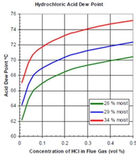
Hydrochloric Acid Dew Point as a function of the concentration of HCl and moisture in Flue Gas.
