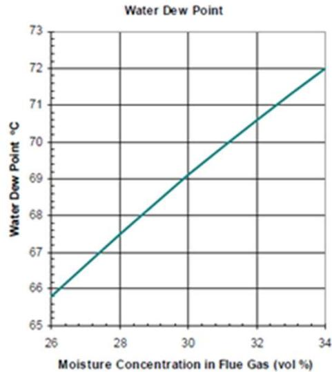
Water dew point as a function of moisture in flue gas.
