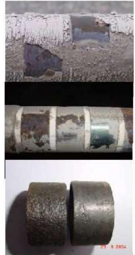
Isolated test material samples situated in the head of a probe. Probe installed thru the wall near super heater combustion gas flow. Test material samples are isolated from each others and they have been wired with fibreglass isolated cable to the termination box in the other end of a probe.
