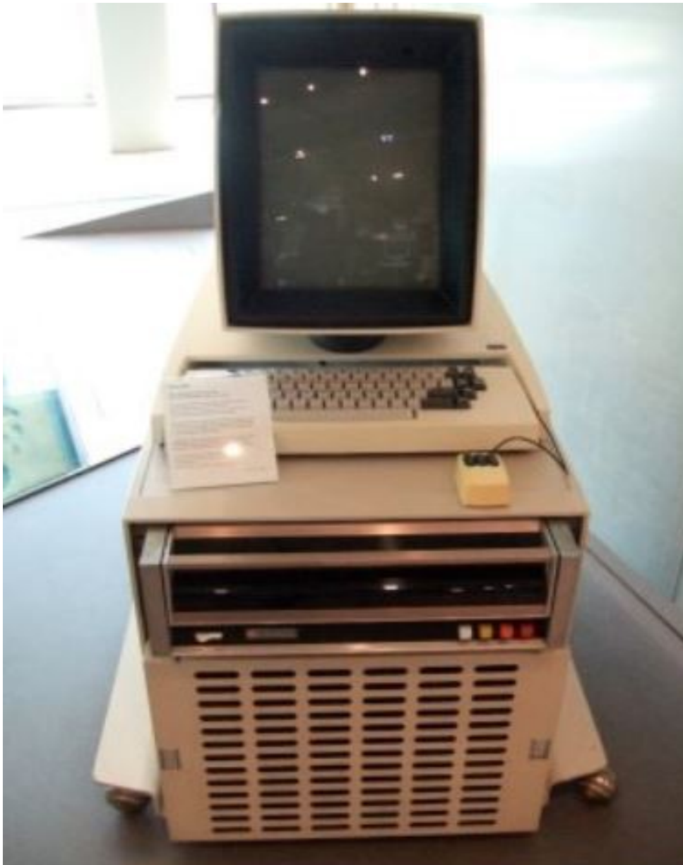
The Xerox Alto computer pioneered many features still used by modern computers today.
