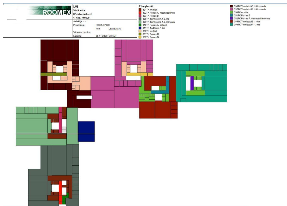
Figure 4.6: Example of the storey-specific ventilation service area chart of the same building; here the presentation method is 2D.
