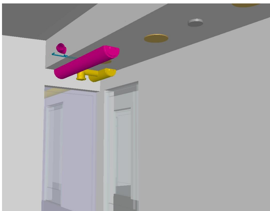
Figure 8.5: Example of modeling that is not permitted. Either the ventilation ducts must be hoisted up, or the suspended ceiling must be lowered.
