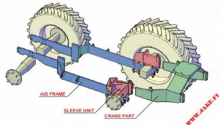
4. When the Crane Part is loose, take a heavy load in the grapple, for instance a heavy log, and stretch the crane boom straight backward to its full outreach. Set the grapple and its load against the ground so that the grapple can not tip over while the crane is parked without the tractor.
