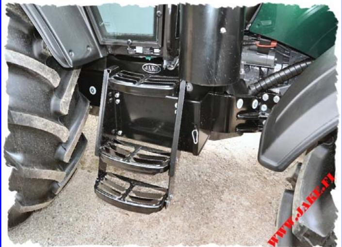
Original battery case is replaced with armoured and lockable JAKE Battery box which is fastened to the Armour (or Aid Frame when Mounting Kit).
