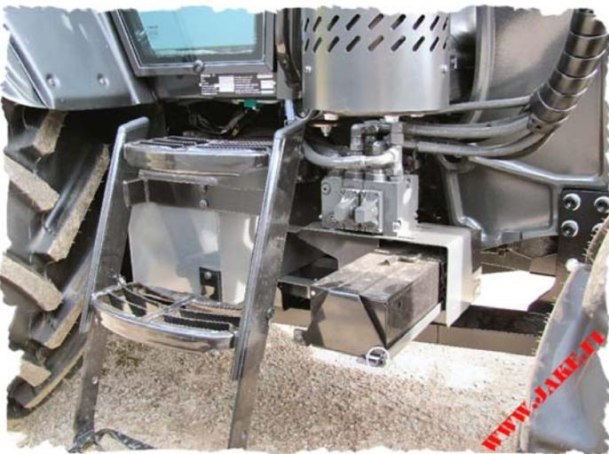
Original battery case stays original and it is not armoured. Armour is fastened partly to the battery case fasteners.
