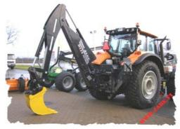
Basically the JAKE D114 uses the hydraulics of the tractor. For fluent use the tractor pump should make around 80 litres of oil per minute at 180-200 bar. The maximum oil pressure for the JAKE D114 is 230 bar which is possible to obtain with a PTO pump. The PTO pump set includes an oil tank integrated into the JAKE D114 frame and an oil cooler. The pump produces 100 litr/min at 1500 rpm of an engine speed.
