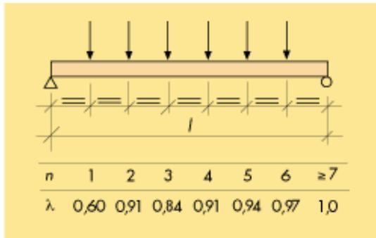
Table 4.2. Effective beam length  $l_e$  in relation to total beam length. Simply supported beam, restrained from buckling at supports and loaded with  $n$  equal loads. The concentrated loads bear at the top edge of the beam and restrain lateral bending in the beam at the loading points.
