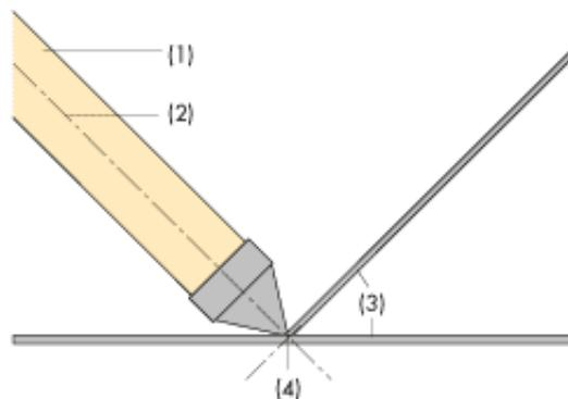
Figure 2.16. System lines should if possible meet at one point, to avoid moments in the node. (1) strut. (2) System line. (3) tie. (4) Theoretical node.
