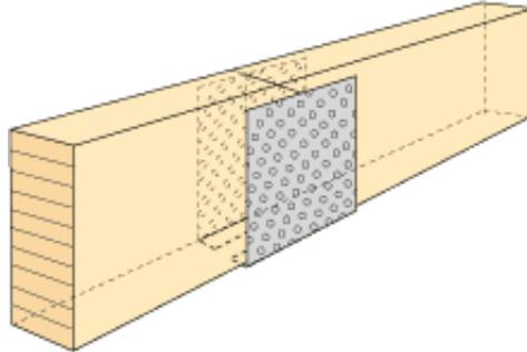
Figure 13.34 Gerber fixture type BMF-W.
