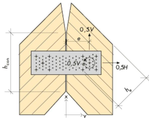
Figure 13.27 Pinned ridge joint with fishplates of nailplate. Symbols.
