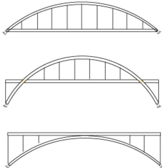
Figure 16.12 Arch bridges with through, half-through and deck roadways.
