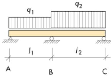
Figure 6.1. Continuous beam on three supports
