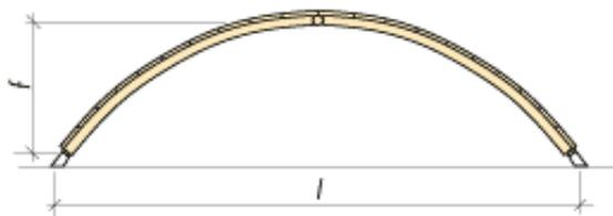
Figure 10.2 Arch springing from foundations.
