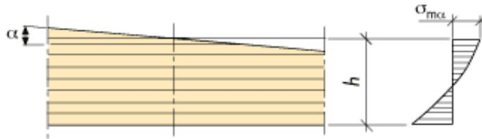
Figure 6.4. Distribution of bending stresses in beam of varying depth
