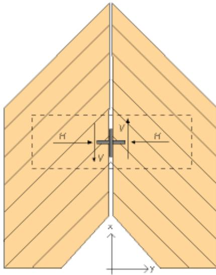
Figure 13.29 Cruciform connector of welded flat steel. Symbols.
