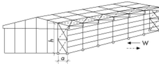
Figure 12.1 Bracing of glulam structure using wind trusses and wall bracing.
