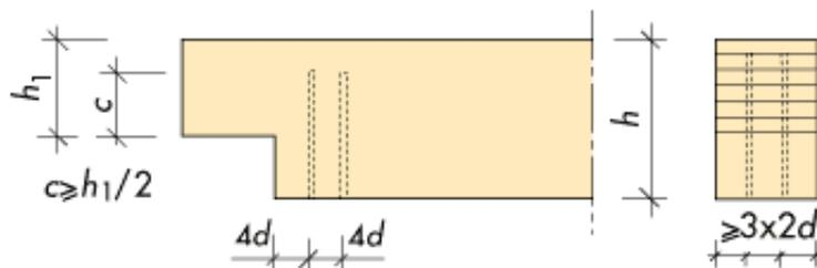
Figure 4.9 Notch in beam end. Reinforcement with glued-in screws.
