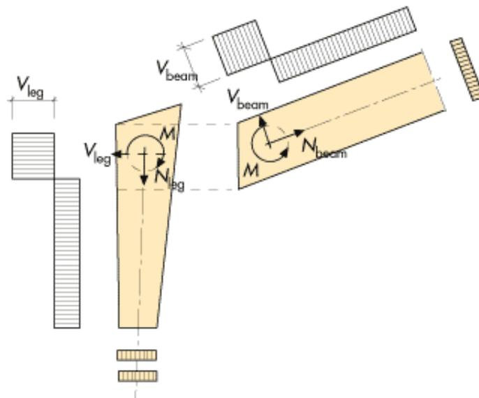
Figure 9.8 Cross-section forces and lateral force diagram for frame beam and frame leg.
