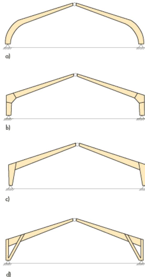
Figure 9.1 Examples of designs of three-pin portal frames
