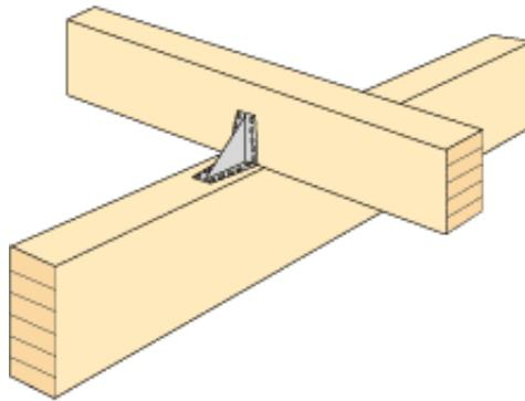
Figure 13.36 Fixing purlins with angle of cold-formed steel.
