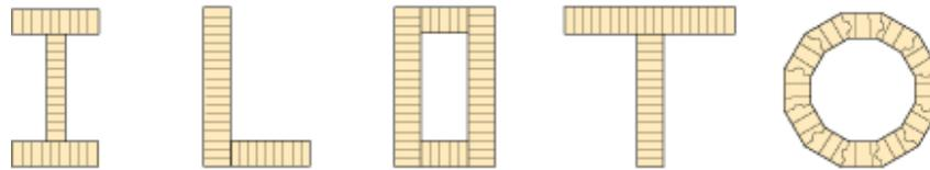
Figure 1.10 Examples of composite glulam sections.
