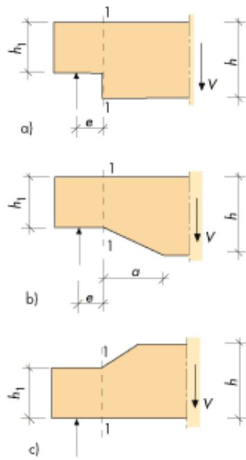
Figure 4.6. Notches in beam end. Symbols.
