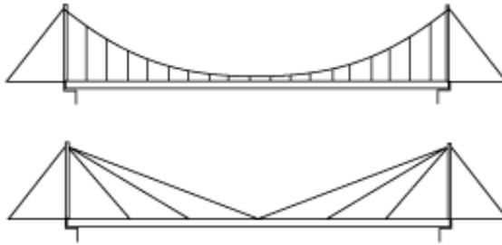
Figure 16.3 Suspension bridge and cable stayed bridge.
