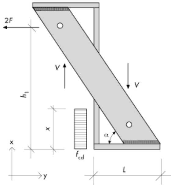
Figure 13.33. Welded Gerber fixture. Symbols.
