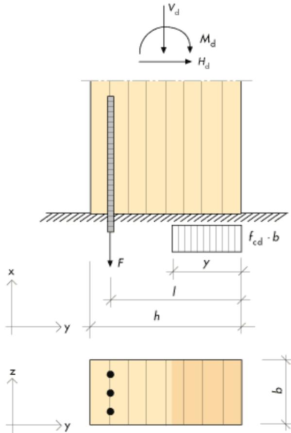
Figure 13.13 Rigidly fixed column base with glued-in bolt. Calculation model.
