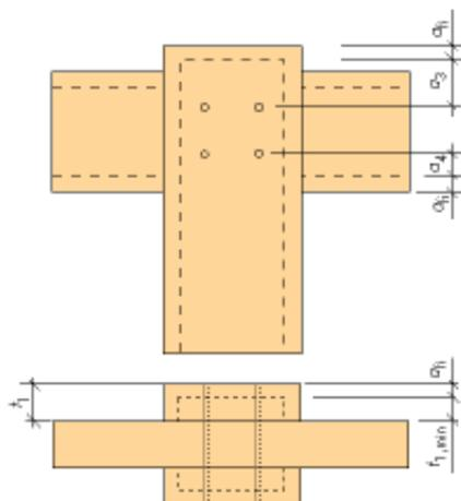
Figure 14.2. Increased sizes of unprotected joints for fire classes higher than R15.
