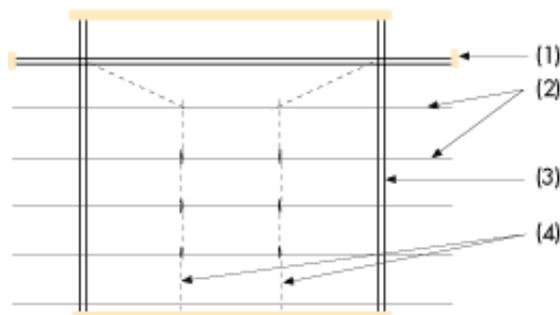
Figure 11.4 In steep roofs the other purlins can be hung up from the ridge purlin. (1) ridge purlin; (2) Other purlins; (3) Roof beam; (4) Suspension rod.
