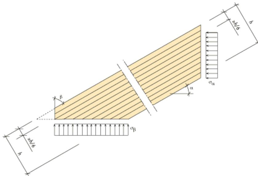
Figure 4.5. Contact pressure at sharp corners.
