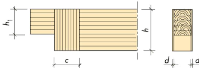
Figure 4.8 Notch in beam end. Plywood reinforcement .
