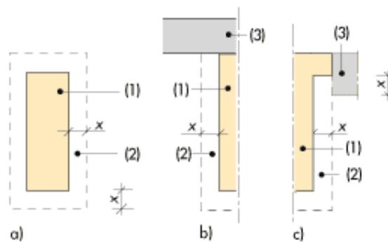
Figure 14.1 Effective residual section after fire (1) original section (2) To the left: Four sided fire exposure. Centre and to the right: Three sided fire exposure, where the top is protected by material with better fire resistance (3).
