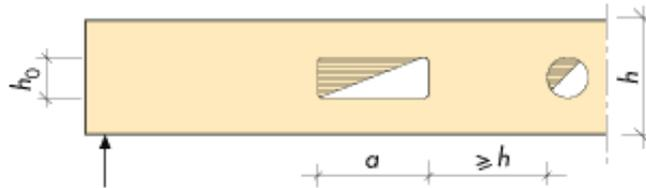
Figure 4.10. Holes in glulam beams. Symbols.
