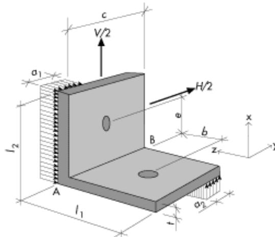
Figure 13.4 Fixture of steel angle. Symbols.
