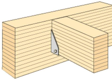
Figure 13.37. Pinned connection between secondary and primary beam with welded hanger. Principle.
