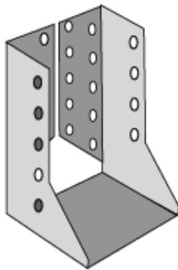
Figure 14.9 Hanger with bent-in flaps.
