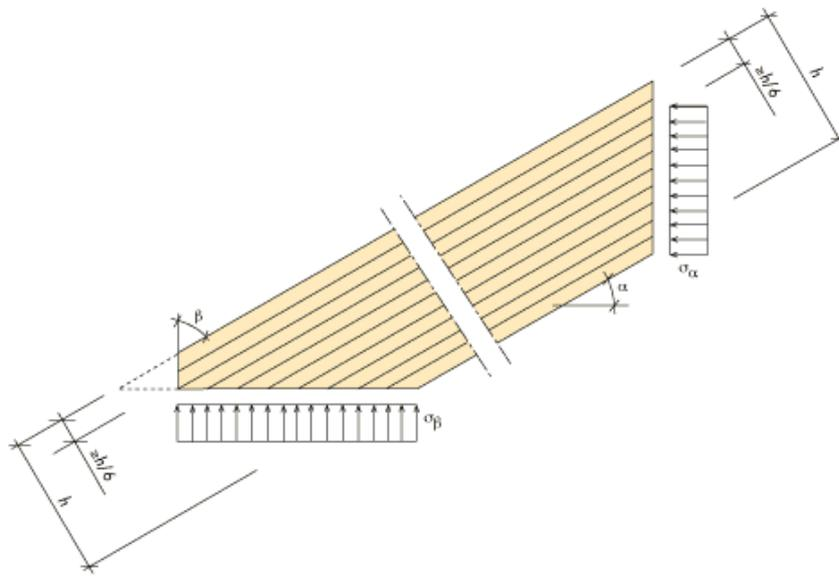
Figure 4.5. Contact pressure at sharp corners.
