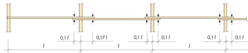
Figure 11.1 Continuous purlin system with overlaps.
