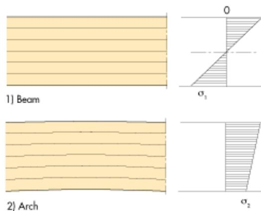
Figure 2.10 Bending stresses in a loaded beam (1) vary through the depth. Compression at the top and tension at the bottom. At the centre of the cross section the stress = 0. An arch (2) on the other hand has compression throughout its cross-section.
