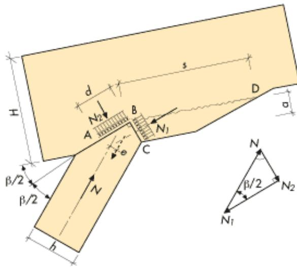
Figure 9.10 Framed joint. Force distribution and symbols.
