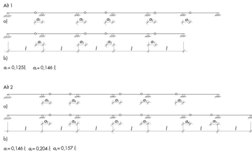
Figure 11.2 Various types of Gerber system.
