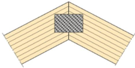
Figure 13.26 Pinned ridge joint with fishplates of nailplate. Principles.
