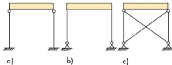
Figure 12.2 Examples of structures which are stable in their own plane.
