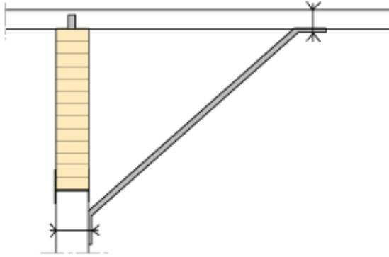
Figure 13.24 Side bracing of column top.
