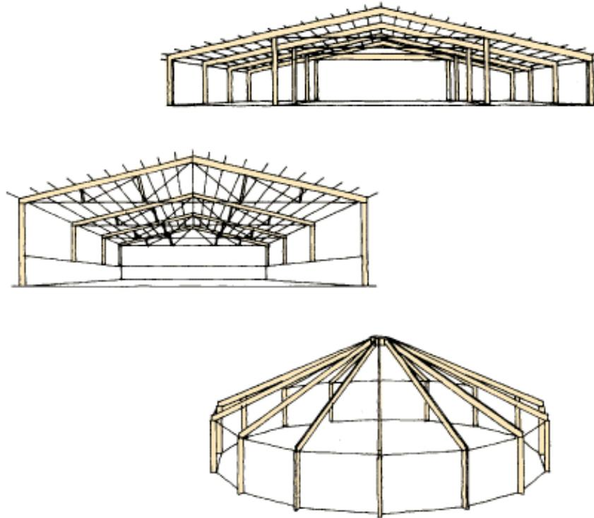
Figure 2.7 Three-pin trusses.
