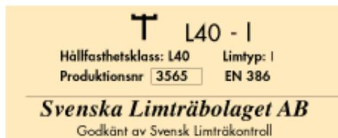
Figure 1.9 Examples of marking.
