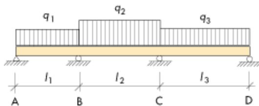
Figure 6.2. Continuous beam on four supports
