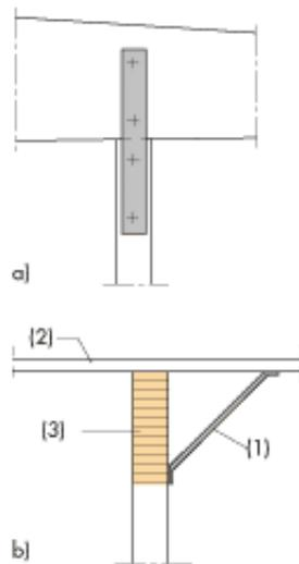
Figure 4.1 Lateral restraint at intermediate support. a) with U-section or heavy fishplate. b) with diagonal bracing. (1) from purlin (2) to bottom edge of beam.
