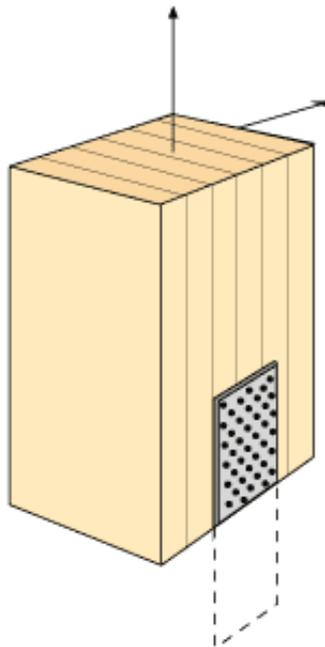
Figure 13.1 Pinned fixing of column foot with fishplates of nailplate. Principle sketch.
