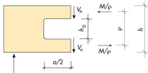
Figure 4.12 When designing rectangular holes it is necessary to take into account the effect of the moment caused by the shear force.
