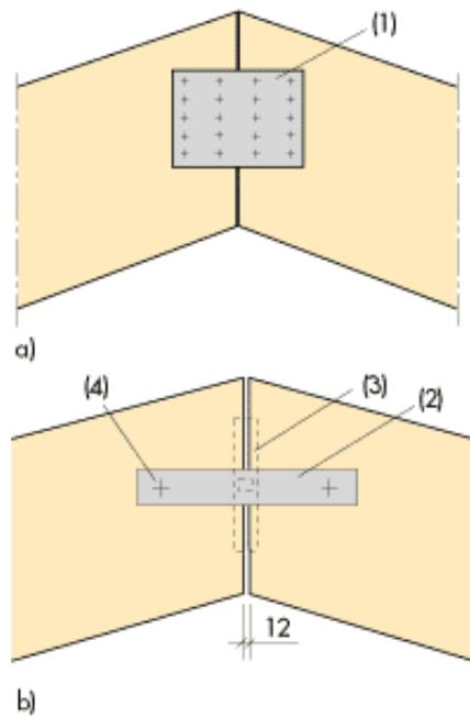
Figure 14.14 Ridge joint a) Nailplates (1): fire protection must be applied. b) BMF-type ridge fixture (3) steel flat (2) bolt (4) R30
