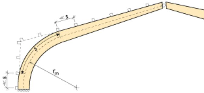
Figure 4.3 Buckling at a curved frame haunch. Symbols.
