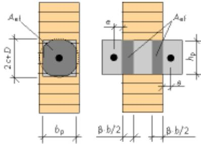
Figure 13.40. Effective contact area with one or two tie rods. Symbols.
