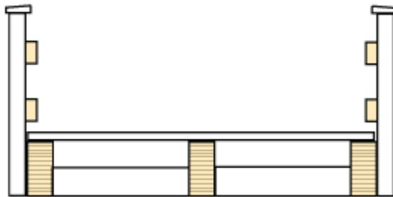
Figure 16.5 Girder bridge with planks laid direct on the glulam beams.
