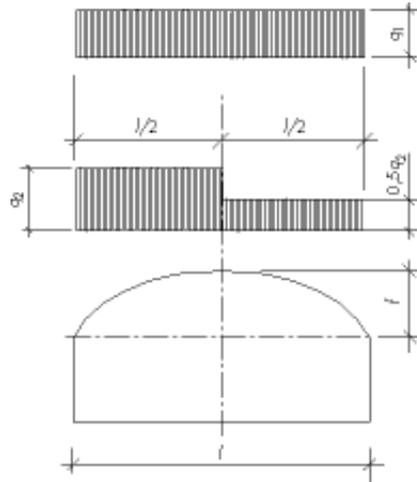
Figure 10.4 Example of various load distributions on an arched roof.
