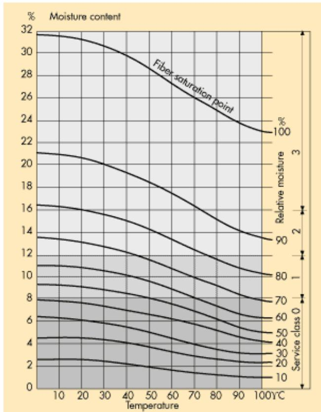
Figure 3.1 Equilibrium moisture content in timber as a function of the temperature at different levels of vapour pressure.
