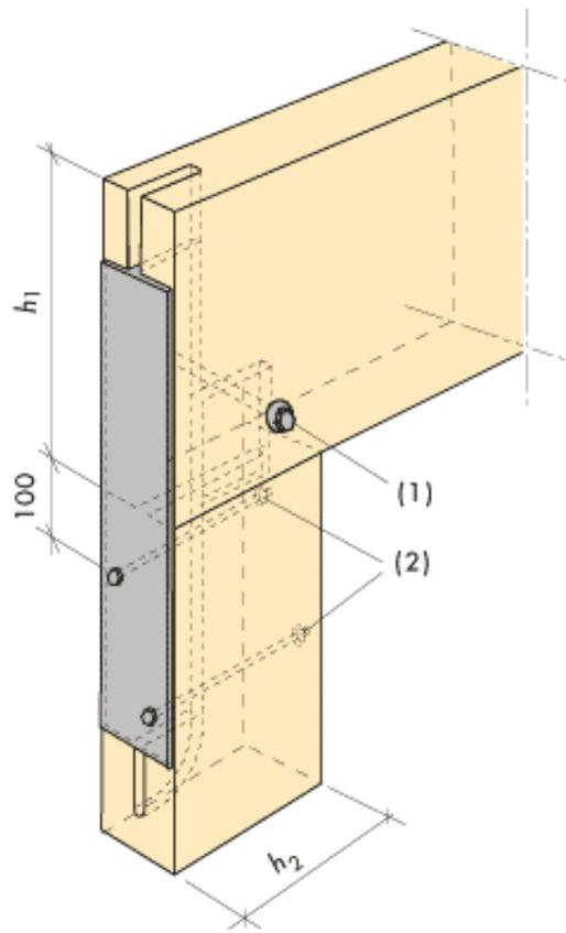
Figure 14.7. Connection column-beam with slotted-in T-section: R30-R60.
