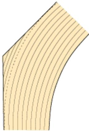
Figure 9.4. Curved haunch with fully glued corner piece.
