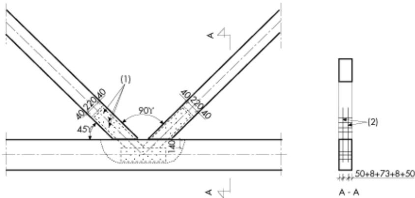
Figure 7.3 Example of design of node in a long-span truss
