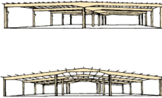
Figure 2.4 Continuous beams.
