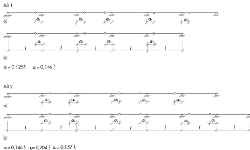
Figure 11.2 Various types of Gerber system.
