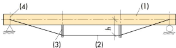
Figure 2.8. Example of bottom-tensioned beam with a constructional height of  $h$ . (1) beam. (2) tension member. (3) compression member (4) recessed or external steel fixtures.
