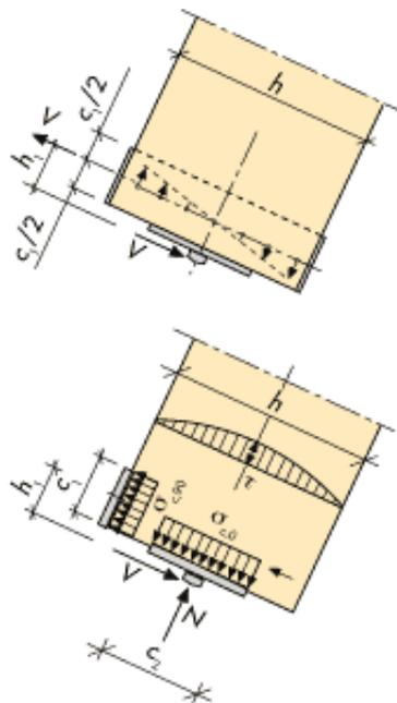
Figure 13.45. Transfer of forces between fixture and glulam. Calculation models.
