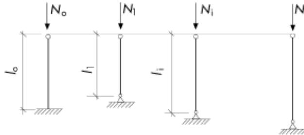
Figure 5.5 Column system with one rigidly fixed column.
