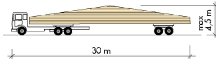
Figure 1.13. If the length of the vehicle exceeds 30 m police escort is usually required.
