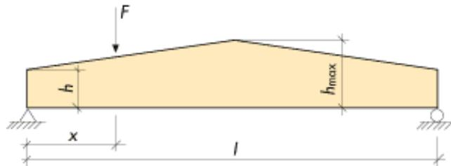
Figure 6.6 Simply supported, double tapered beam with concentrated load.
