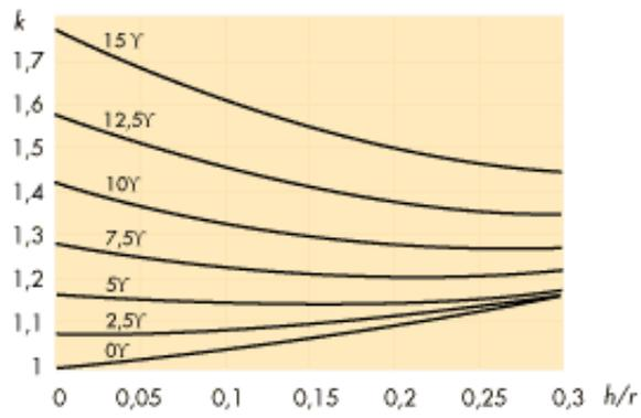
Figur 6.8 Coefficient  $k_f$  for curved beam with varying depth and with different roof slopes and curvature.
