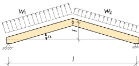
Figure 8.2 Three-pin truss with simple roof beams and tension member. Upward load.
