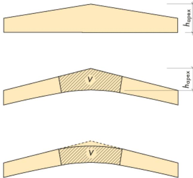
Figure 4.15 Double tapered beam, pitched cambered beam and curved beam with constant depth.
