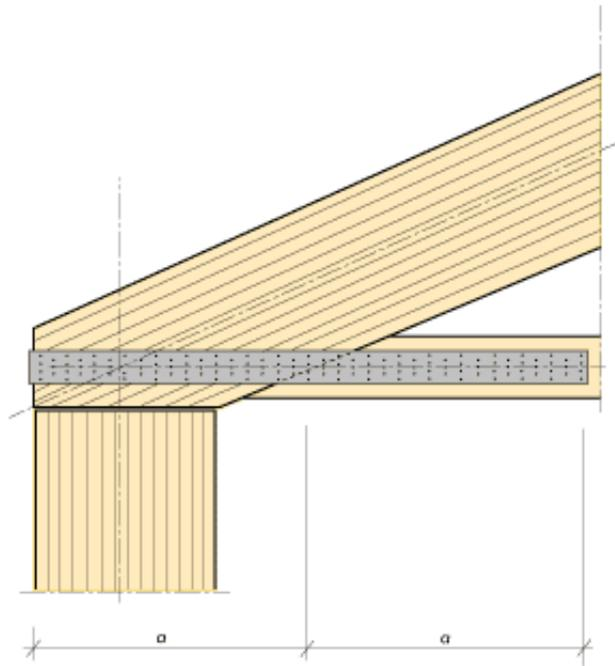
Figure 13.41 Fixing of glulam ties. Principles.
