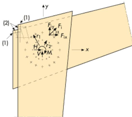
Figure 9.7 Bolted frame haunch. Symbols.
