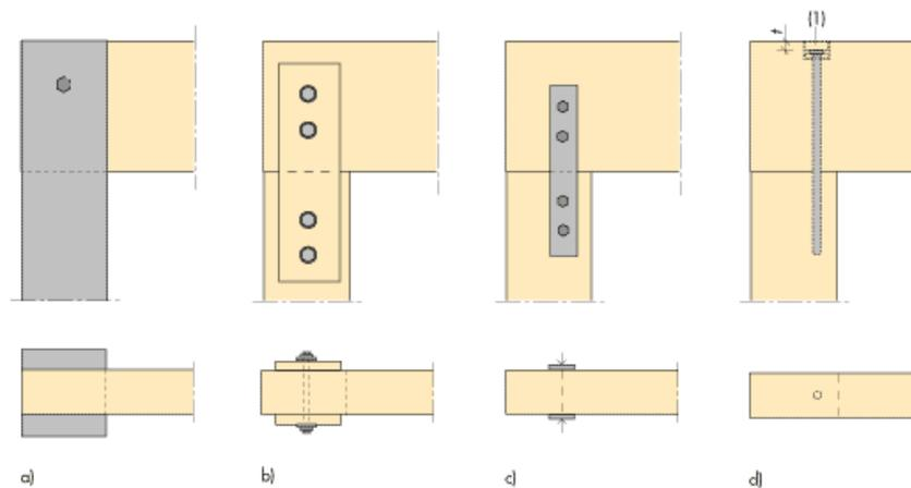
Figure 14.6. Connection between column and beam. a) Concrete fork: R60. b) Glulam fork: R30-R60. c) Steel flats: R30. d) Glued-in screw: R30-R60.
