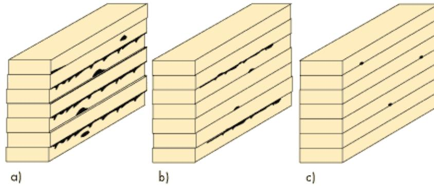
Figure 1.11 Appearance grades, examples. a) equalized surfaces b) industrial appearance grade c) architectural appearance grade
