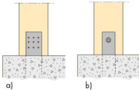
Figure 14.3 Pinned fixing of column base. a) Cast-in nailplate: R60. b) Cast-in flat steel and screw/bolt: R60.
