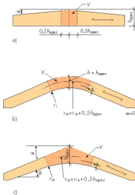
Figure 6.7. Curved beams with constant and varying depths. The characteristic volume  $V$  is marked in the figure.
