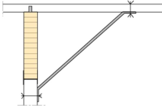
Figure 13.24 Side bracing of column top.
