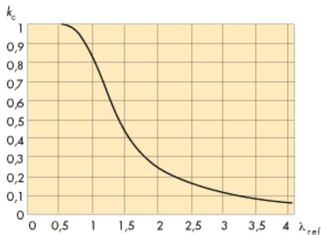
Figure 5.3 Reduction factor  $k_c$  as a function of the relative slenderness ratio according to EC5.
