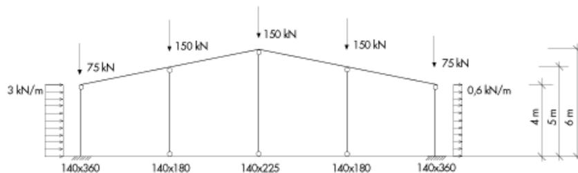
Figure 5.6. Conditions for the calculation example.
