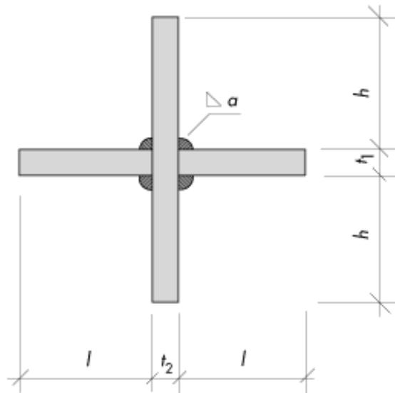
Figure 13.28 Cruciform connector of welded flat steel for transfer of shear forces.
