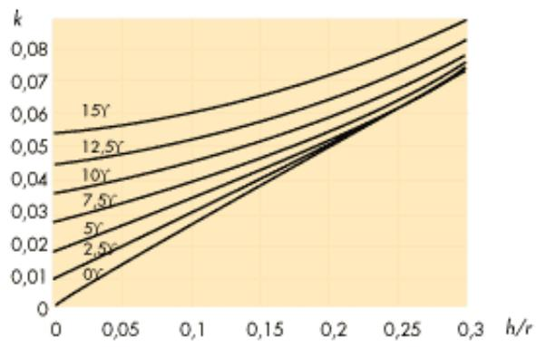
Figure 6.9 The coefficient  $k_p$  for curved beam with varying depth and with various roof slopes and curvature.
