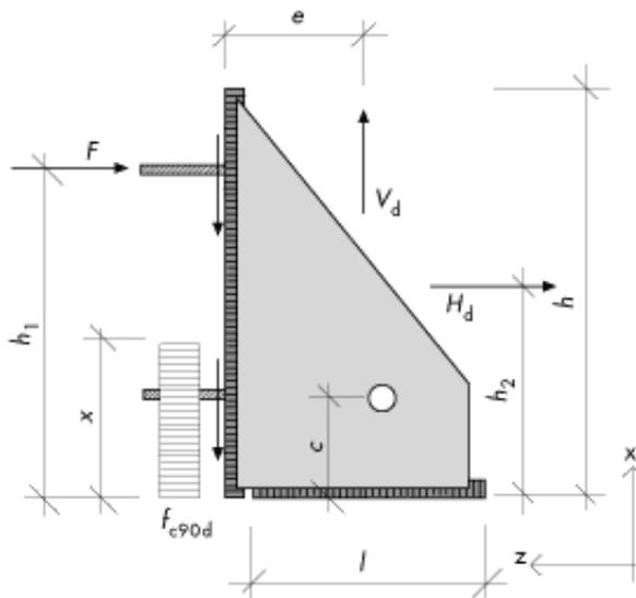
Figure 13.38 Welded beam hanger. Symbols.
