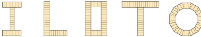
Figure 1.10 Examples of composite glulam sections.
