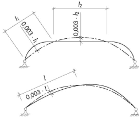
Figure 10.5 Example of an assumed initial deformation under symmetrical and unsymmetrical loadings.  $l$ ,  $l_1$  and  $l_2$  are the distances between points which have not moved during the deformation of the arch.
