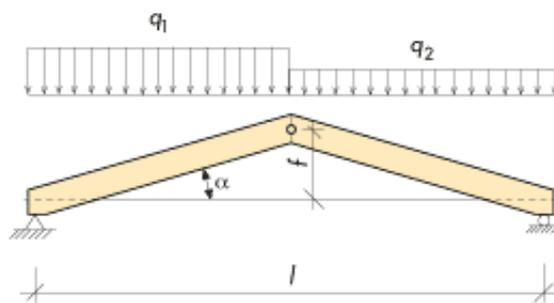
Figure 8.1 Three-pin truss with simple roof beams and tension member. Downward load.
