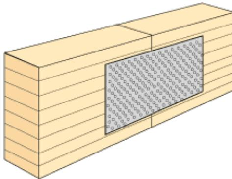
Figure 13.31. Pinned beam joint with fishplates of nailplate. Principles.
