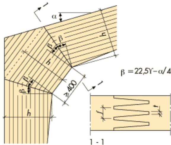
Figure 9.5 Finger jointed haunch with jointing piece.
