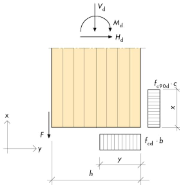
Figure 13.11. Rigid fixing with fishplates. Calculation model with compression stress blocks. Symbols.
