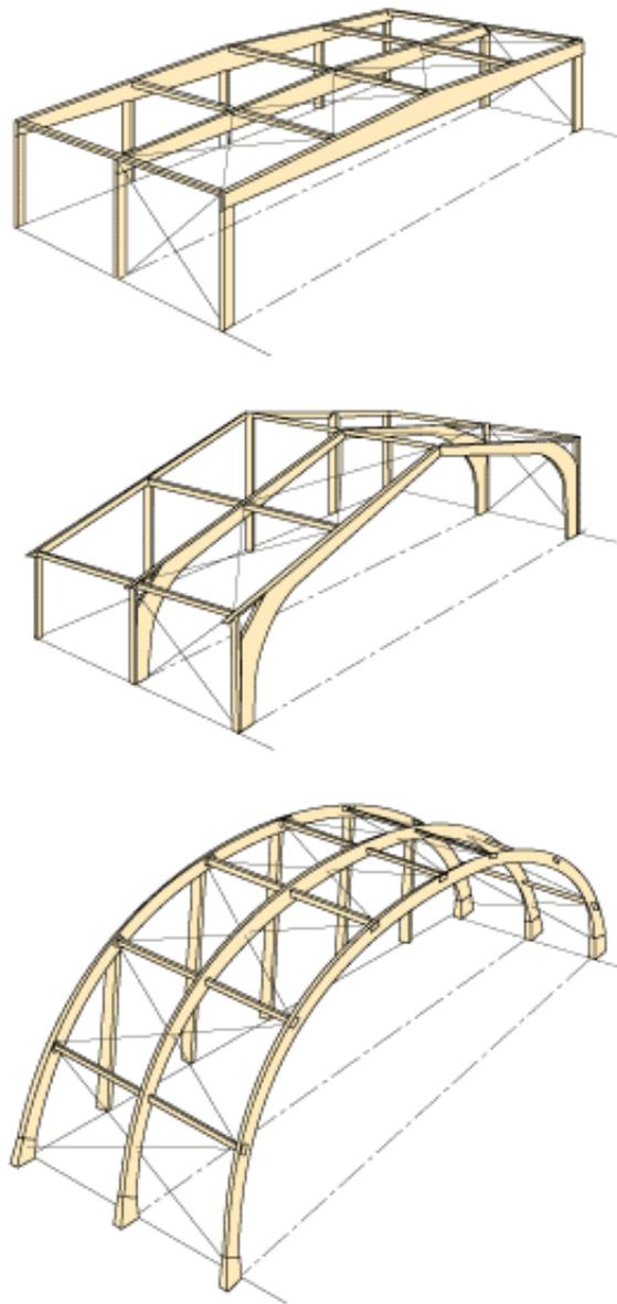
Figure 12.3 Wind bracing of frame and arch structures.
