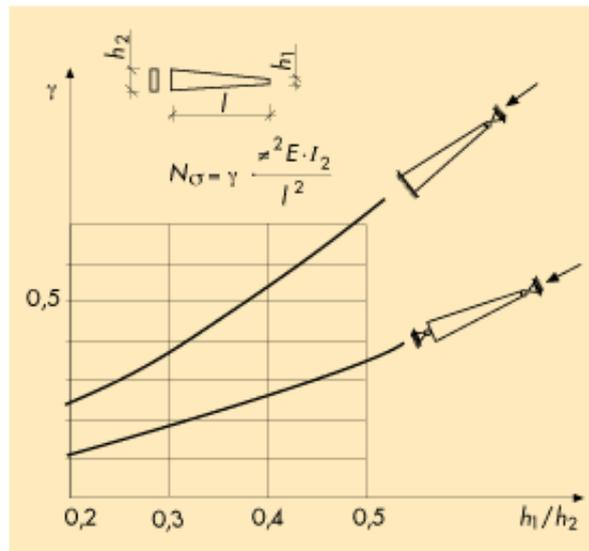
Figure 5.2 Diagram for determining the buckling load of columns whose cross-sectional depth has a linear variation.
