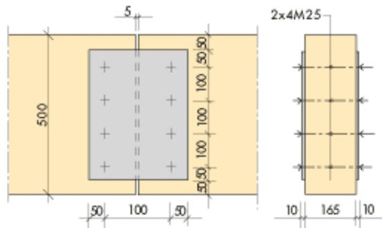
Figure 14.12 Bolted beam joint: R30.
