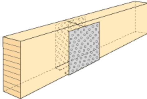
Figure 13.34 Gerber fixture type BMF-W.
