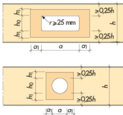
Figure 4.13. Plywood reinforcement of hole. Symbols.
