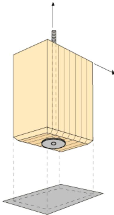
Figure 13.7 Pinned fixing of column base with glued-in bolt. Principle.
