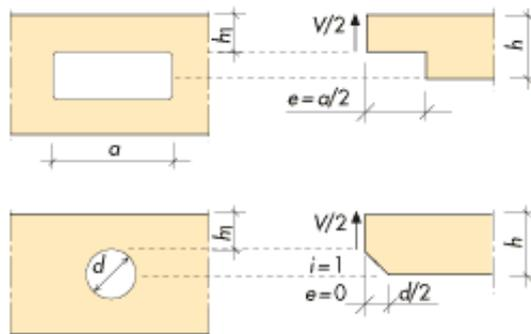
Figure 4.12 Analogy between holes and notches at the end of a beam. Symbols.
