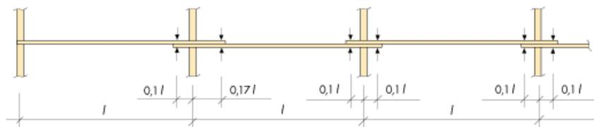
Figure 11.1 Continuous purlin system with overlaps.
