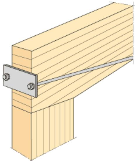
Figure 13.39 Fixing of steel tie. Principle.
