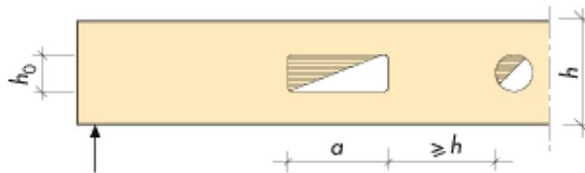
Figure 4.10. Holes in glulam beams. Symbols.
