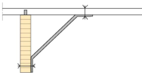
Figure 13.25 Bracing of continuous beam.
