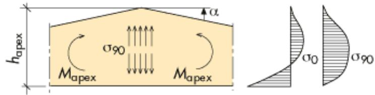
Figure 6.5 Distribution of bending stresses and tension stresses perpendicular to the grain at the ridge of a double tapered beam.
