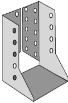
Figure 14.9 Hanger with bent-in flaps.
