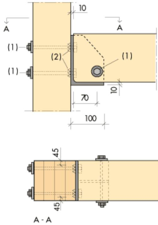
Figure 14.11. Beam connection with steel bracket and screws/bolts with connectors: R30.
