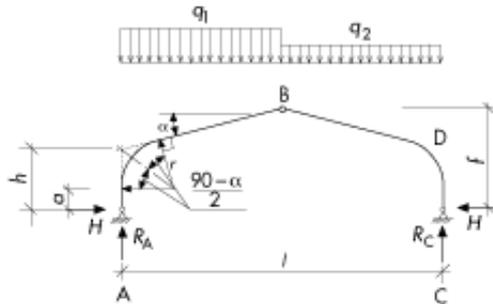
Figure 9.2 Three-pin frame with curved haunches. Symbols.
