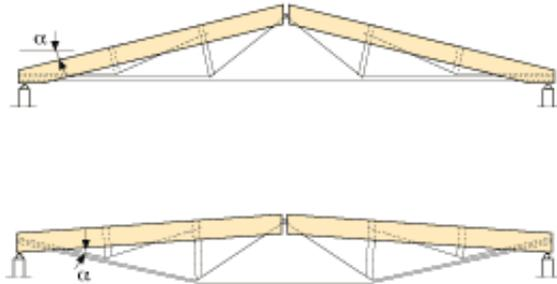
Figure 8.4 Three-pin truss with timber struts and steel ties.
