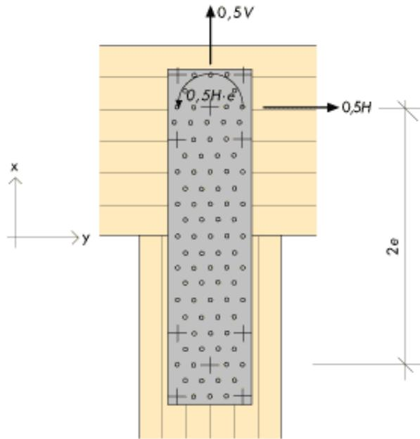
Figure 13.19. The fishplate is regarded as a beam rigidly fixed at both ends. Symbols.
