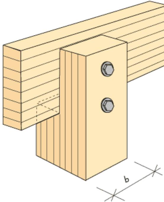
Figure 13.22 Pinned connection between beam and column with the beam recessed in the top of the column. Principles.
