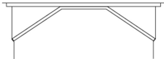
Figure 16.11 Example of a simple strut frame.
