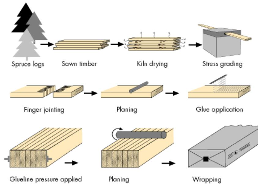
Figure 1.2 Glulam manufacture. Schematic.
