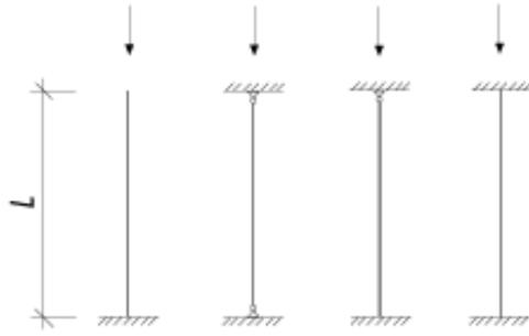
Figure 5.1 Various end conditions in buckling
