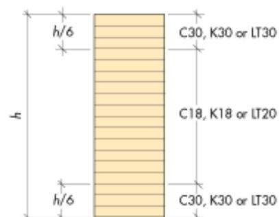
Figure 1.3 Lay-up of combined glulam
