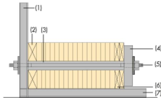
Figure 1.4. Schematic section through gluing bench. (1) Vertical stop. (2) Pressure distributing base, possible camber pattern. (3) Distance piece. (4) Compression block. (5) Tension screw. (6) Pressure distributing boards. (7) Horizontal stop.
