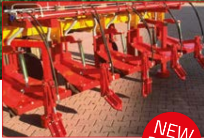
4-row ridger, type 'Super' (ZR4) with hydraulic anti-erosion flaps (RS1054)
