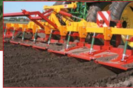
Ridging – ridging with dividing discs and V-puller before crops emerge (RS75)
