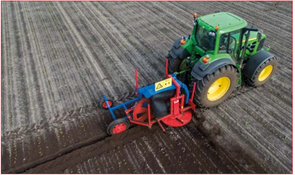
ZIBO ditch digger with horizontal adjustable disposable disc (SF0335) and support wheel (SF0615)
