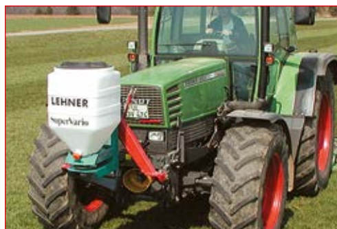
Multifunctional Lehner Super Vario® Universal centrifugal spreaders
