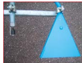
2 types distributors: point distributor (left) (GS0146) V-distributor (right) (GS0131 or GS0132)
