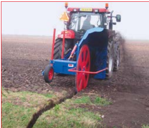
ZIBO ditch digger with support wheel (SF0315) and hydraulic depth control (SF0316)
