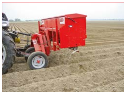
ZZ2603 ZIBO fertilising unit fitted with hitch with weighing installation
