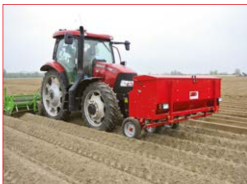
ZZ2603 ZIBO fertilising unit fitted with hitch with weighing installation
