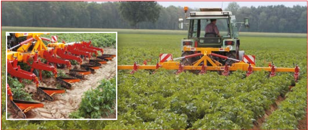
Insert: ZIBO hoebalk 8 row with ZIBO Super anaarders with edging boards
