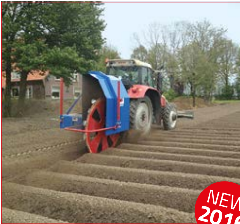
ZIBO ditch digger (SF0501) with mirrored frame
