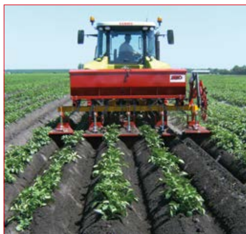
ZIBO ridger (ZR4) with fertilizer unit (XL26008)
