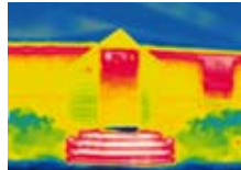
Building: Heat Loss
