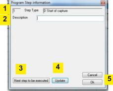
Steps added to the step list contain settable data that must be set before using the program. The setting is done by selecting a row or a step from the step list. Double-clicking or the "Enter" button opens the "Step data" dialogue, in which the values are set. The settings to be changed vary according to the step type. Fields that are common for all step types are as follows (Picture above):
