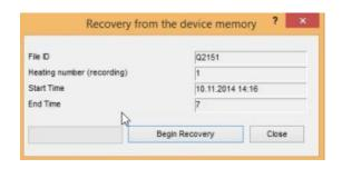
Recovering process data from memory is not possible if earlier "Delete" button is used and memory is empty
