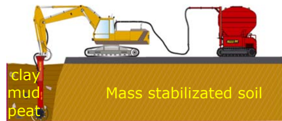
Mixing tool installed on an excavator machine and a binder storage tank 15
