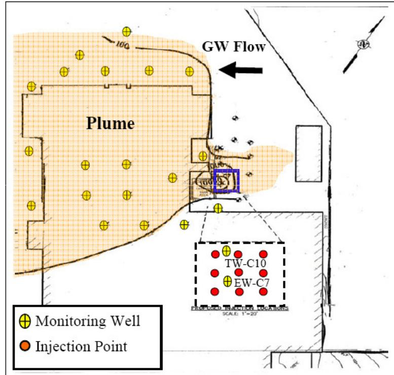
Figure 1. Site Map with RegenOx Injection layout
