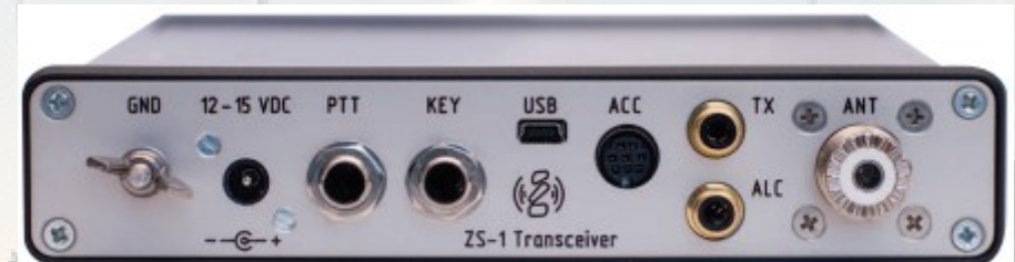
PHOTO 2: Zeus ZS-1 interconnections on the rear panel.
