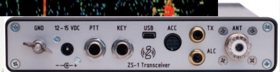
PHOTO 2: Zeus ZS-1 interconnections on the rear panel.
