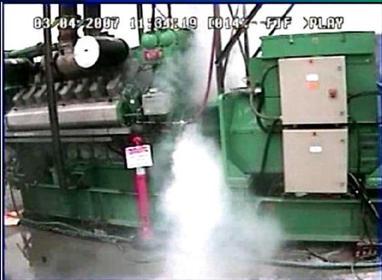
Generator room at the Idaho National Laboratory was remote accessed by a hacker and Million diesel-electric generator destroyed. (U.S. Homeland Security photo)
