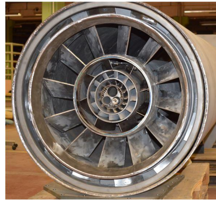
New multi fuel burner
