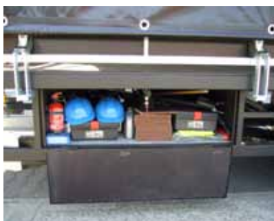
Lockable equipment compartment with basic safety equipment
