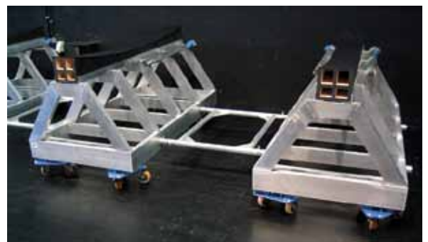
Individual storage trolleys for acoustic elements
