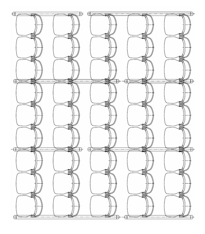
Typical layout principle using 2 and 3 row interconnecting floor bars.
