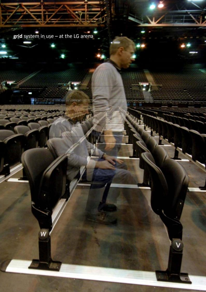
**grid** flat-floor seating system allows any choice of seat tipping model to be arranged in row formation on a flat floor - the **grid system is** lightweight and robust and easy to layout and has the following advantages —
