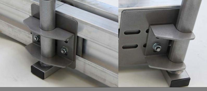
**nomad** seats can be applied to any temporary structure – scaffold systems – frame systems – SPS – our attachment system consists of extruded aluminium profiles to accommodate a 2.5M system span. Steel attachment clamps slide into the extruded profile and can be positioned anywhere so that any system span can be accommodated. Connector assembly's are also available so that profiles can be joined end to end.
