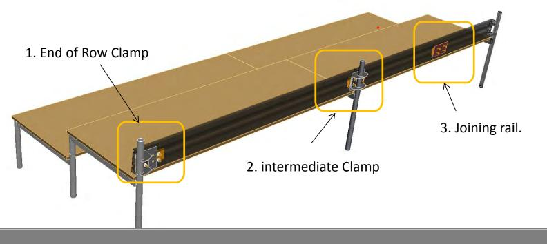
The illustration above shows a typical scaffold based structure with a 2.5 span.
