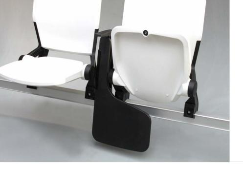
**scribe** has an anti-panic feature so that in an emergency - as the user leaves the seat the tablet will automatically return to the stowed position in a controlled fall - leaving the exit clearway un - obstructed.
