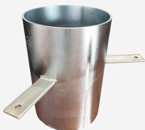
Socket casing. Steel, galvanized. Diameter: 127 or 219 cm. Height: upon request.
