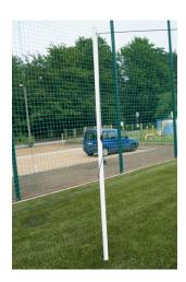
Two tensioning uprights, made of steel tubes [48,3x3,2 mm], painted twice: base, anti-corrosion layer and then powder-coated
