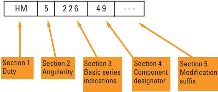
A new inch part numbering system was developed by the American Bearing Manufacturers Association (ABMA) to address the expansion in the number of new applications and tapered roller bearing designs. This part numbering system has become the international standard for inch-sized bearings.
