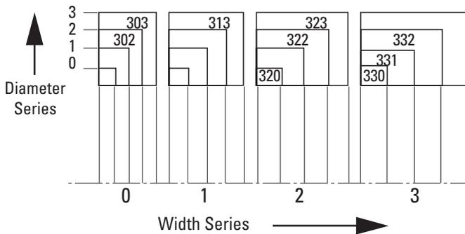
The original metric part numbering system for tapered roller bearings was based on the ISO 15 dimensional plan for radial bearings. A 5-digit part number commencing with numeral 3 describes the bearing assembly (inner race and outer races).
