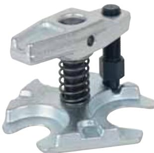
Adjustable ball joint extractors lever type, for all passenger cars, commercial vehicles and medium-sized trucks
