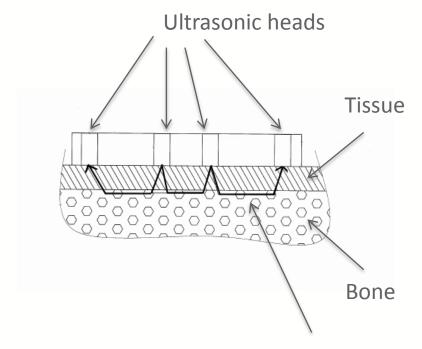
Ultrasound signal travelling in the cortical layer of the bone
