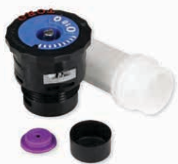
Precision™ Series Spray Nozzle with PCD Nozzle: 12H Nozzle at 50 psi = 0.74 gpm or 1"/hr.*
