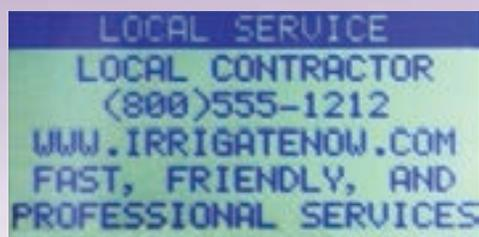
The **Contractor Message Screen** allows the contractor to input a custom message with their name and contact information into the controller from the software via a USB drive so it is visible to the homeowner when they press the "Help" button.
