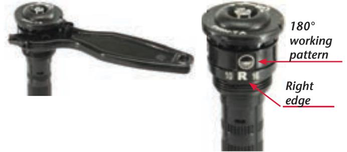
The unique adjustment method allows for pre-setting of arc by hand or tool before the nozzle is installed. Visual indicators allow the user to quickly adjust the arc pattern to the desired arc from 45-270°. The adjustment band can be adjusted by hand or with the pre-included tool.
